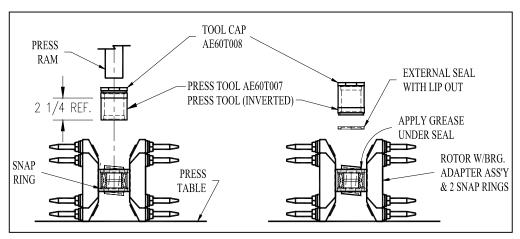
Figure 8. Rotor Assembly
